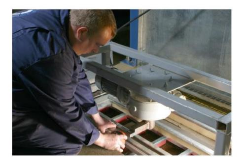
The RSI - Airblast AFC Recovery Floor automatically recovers abrasive material from beneath the operators' feet. A full recovery floor effectively renders the blaster with an endless supply of media, thus eliminating the need to stop production to recover media. The Airflex floor is made of modular corridors of various standard widths that can be produced to any length. Six widths are available, and with this flexibility it is possible to recover from virtually any floor area.
