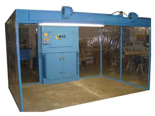
RSI has 2 standard units, one with 9,000 CFM and another with 12,500 CFM, both measuring at 1" static pressure. The 48120 model works great in applications using light and medium sanders with light to medium grit paper. The 85120 model can be used for heavy sanding or even heavy grinding applications done with a very coarse grit paper. This model can be custom made with side openings for use in conjunction with conveyor systems.
